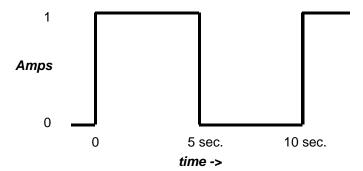
By inspection, the average voltage is 5 volts, and the average current is 0.5 amps. But the average voltage times the average current (= 2.5 watts) is **not** the average power. In fact, that product is meaningless. We need some other measure of voltage and current if we're going to calculate average power without first finding the instantaneous power.
