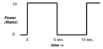
This second waveform of power versus time shows the instantaneous power, that is, the power delivered to the resistor at each instant of time. Too often, it's overlooked that whenever the voltage and/or current varies with time, the power does also. But it's obvious that when the switch is open, no power is being delivered to the resistor. This is extremely important to realize, because it
