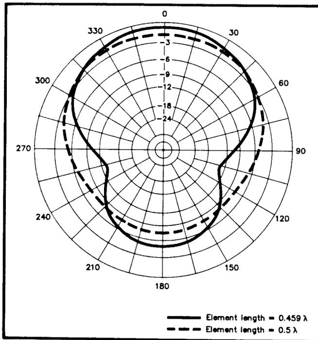
Fig 1—Patterns of two-element arrays fed at the bases with equal currents of 90-degree relative phase. Element spacing is  $0.25 \lambda$ . The two patterns are for antiresonant elements ( $0.459 \lambda$ ) and  $1/2 \lambda$ -long elements above a perfect ground plane. The outer ring of the plot is +11 dBi.
