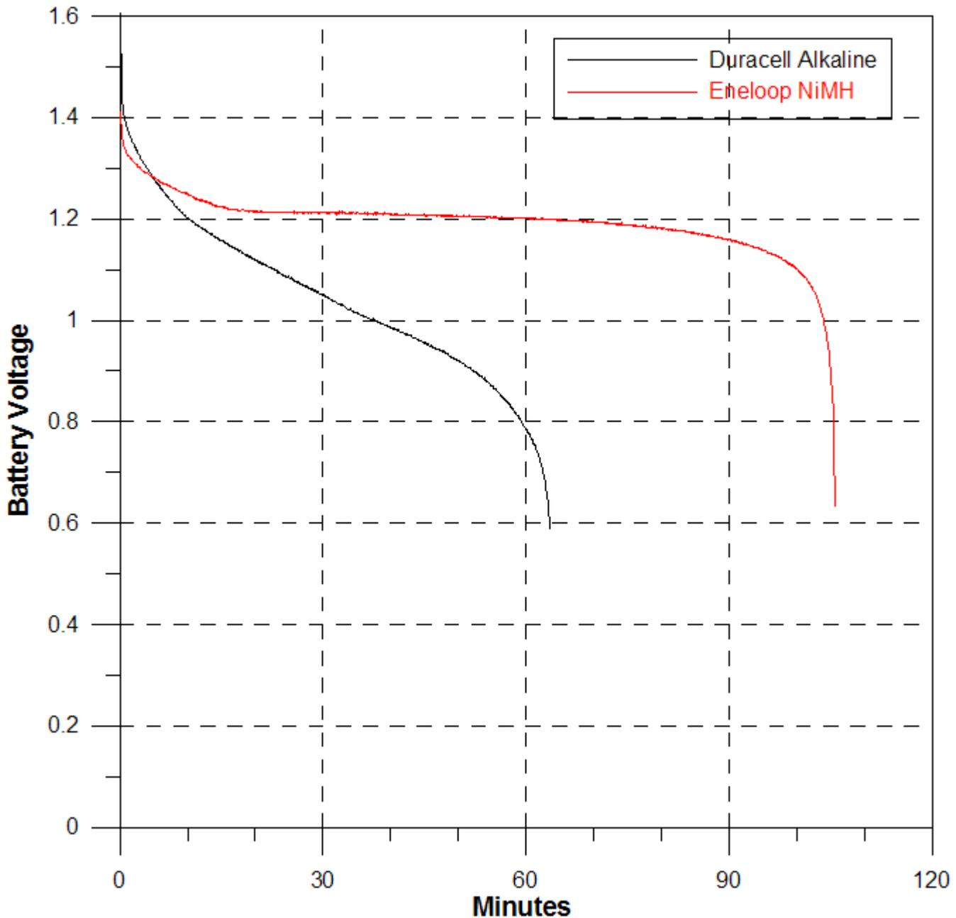
At this current drain, the NiMH cell voltage is higher than the alkaline cell voltage for all but less than the first five minutes. It's interesting to note that the alkaline cell is delivering 1.10 Wh at 1 A, or 69% of the energy it did at 500 mA, but the NiMH cell is delivering 2.10 Wh, or 91% of the energy it did at 500 mA. So while both deliver less total energy with the higher discharge current, the alkaline cell's energy capacity drops much more than the NiMH cell's.
