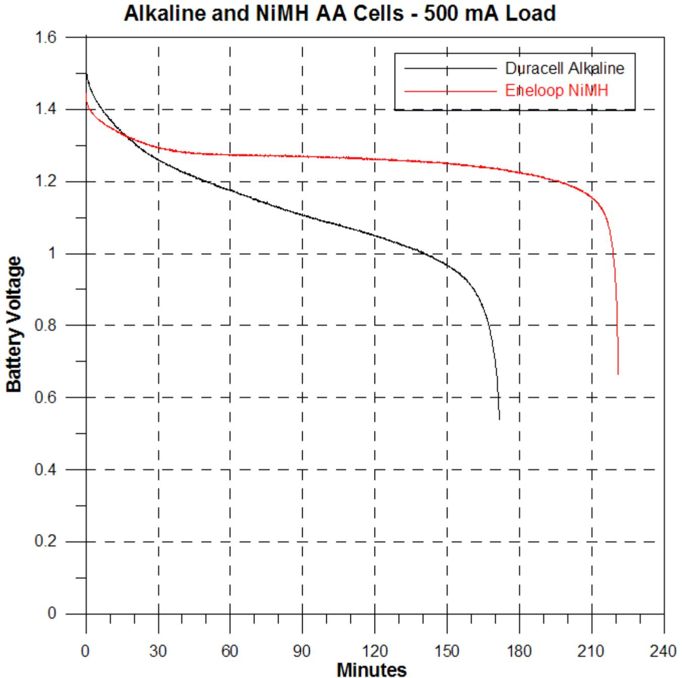
Here we can see that after the first 15 minutes, the “1.2 volt” NiMH cell voltage is higher than the “1.5 volt” alkaline cell voltage! The total energy delivered by the alkaline cell, as noted above, is 1.60 Wh. The NiMH cell is delivering 2.31 Wh.
