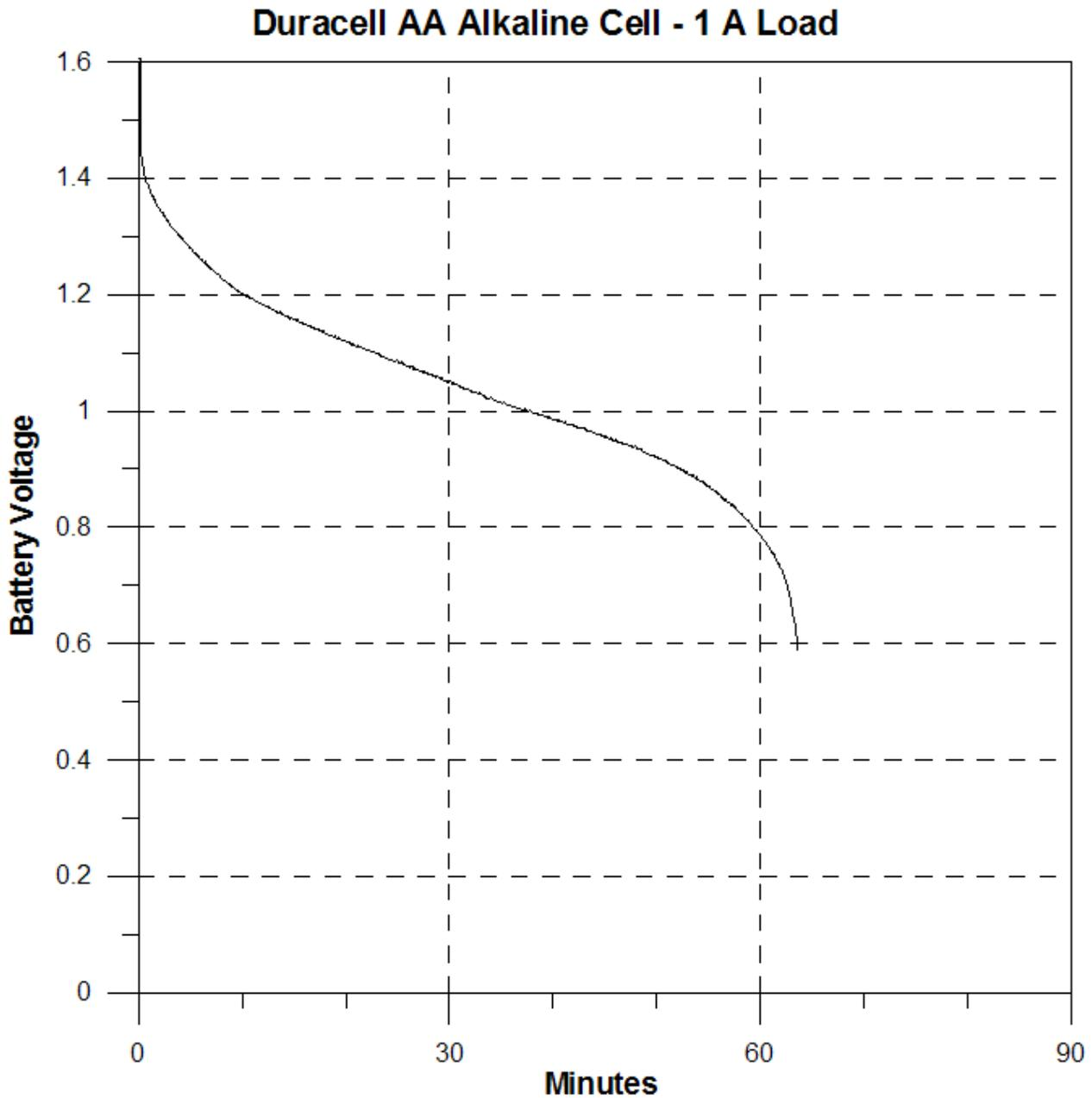
At this discharge rate, the cell voltage is less than 1.2 for all but about the first ten minutes of the hour-long discharge period. This brings us to . . .
