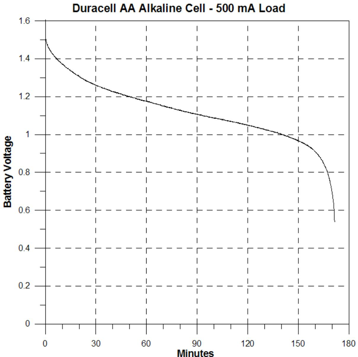
It's obvious from this graph that the “1.5 volt” cell delivers 1.5 volts for only the first few seconds of the discharge. And for the majority of the discharge period, its voltage is less than 1.2 volts.
