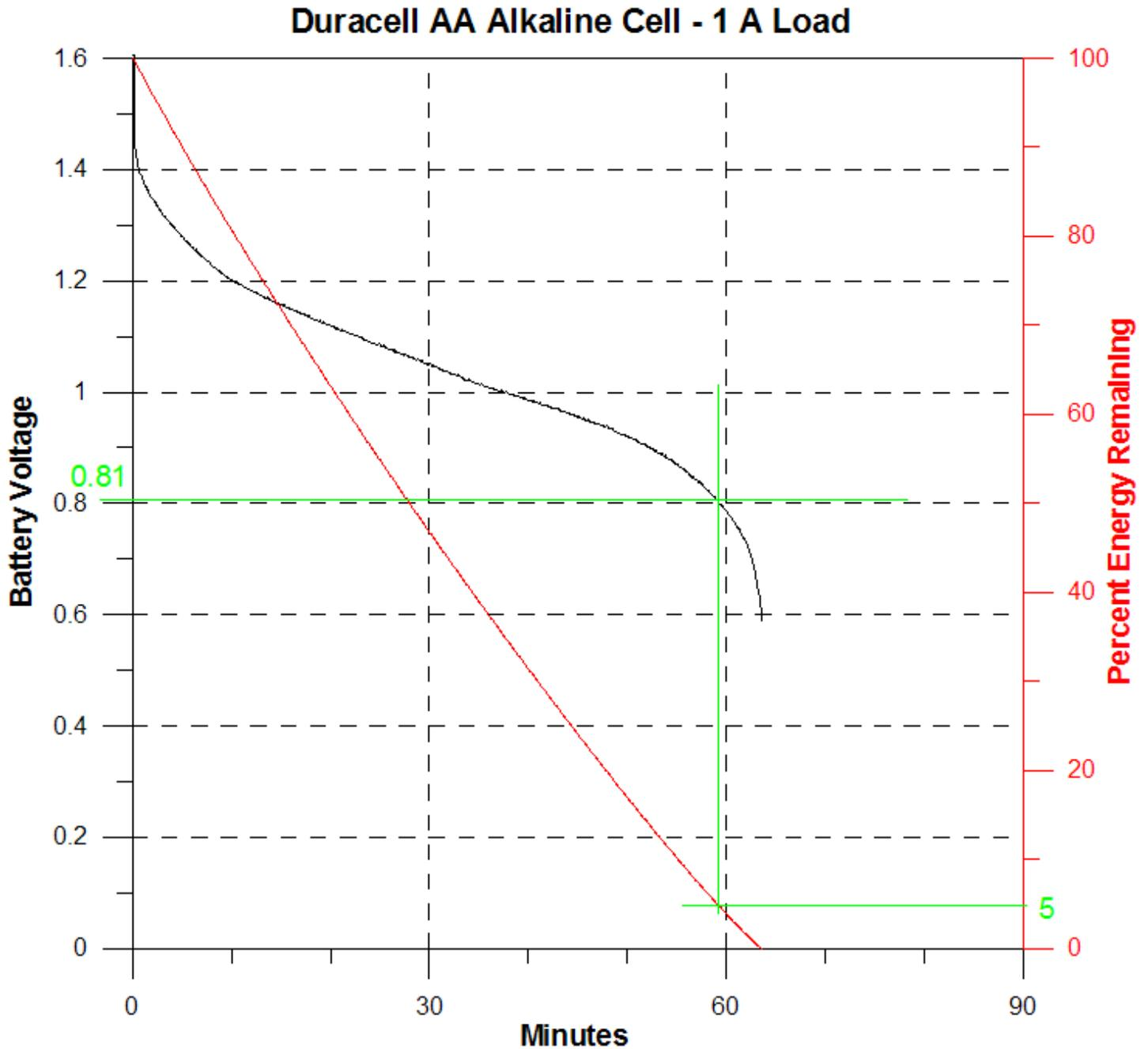
With the higher current drain, only about 25% of the available energy has been extracted when the cell voltage reaches 1.2, and the cell has to be discharged to about 0.8 volt in order to extract 95% of the available energy. Incidentally, the available energy at 500 mA is 1.60 Wh, and at 1 A, 1.10 Wh.
